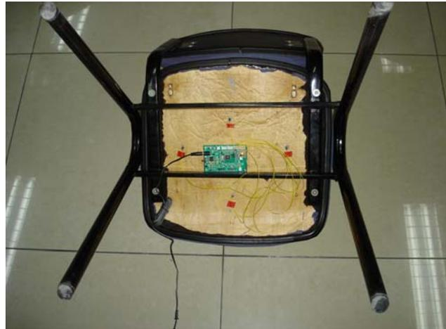
Figure. 17 Slavery MCU and Pressure sensors
